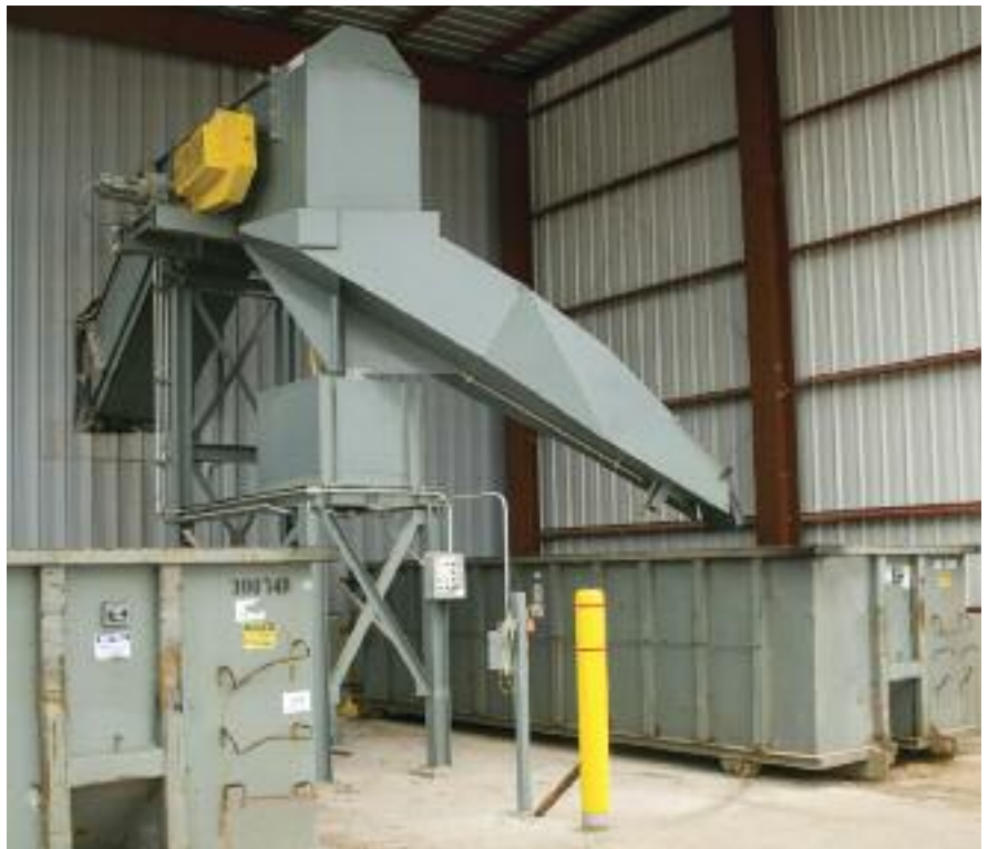
After transport through a below-floor conveyor, scrap is dropped into bins outside of the plant. This chute automatically swivels to empty into a second bin should the first bin become full.
