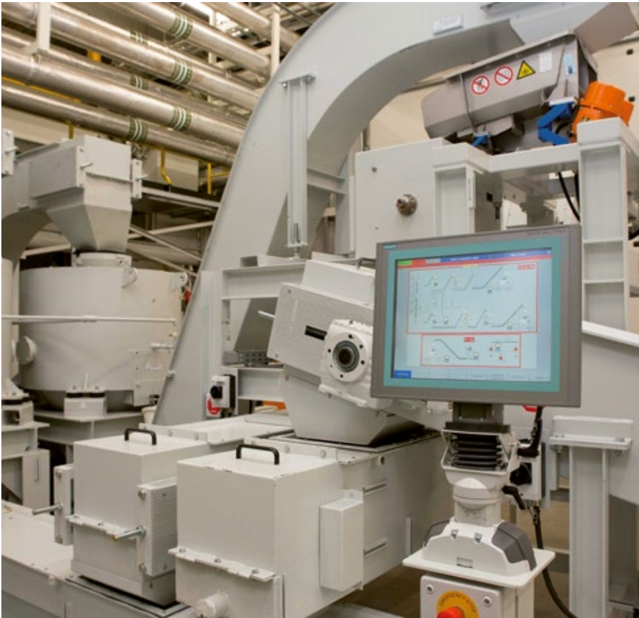
VBU swarf centrifuge for continuous use
