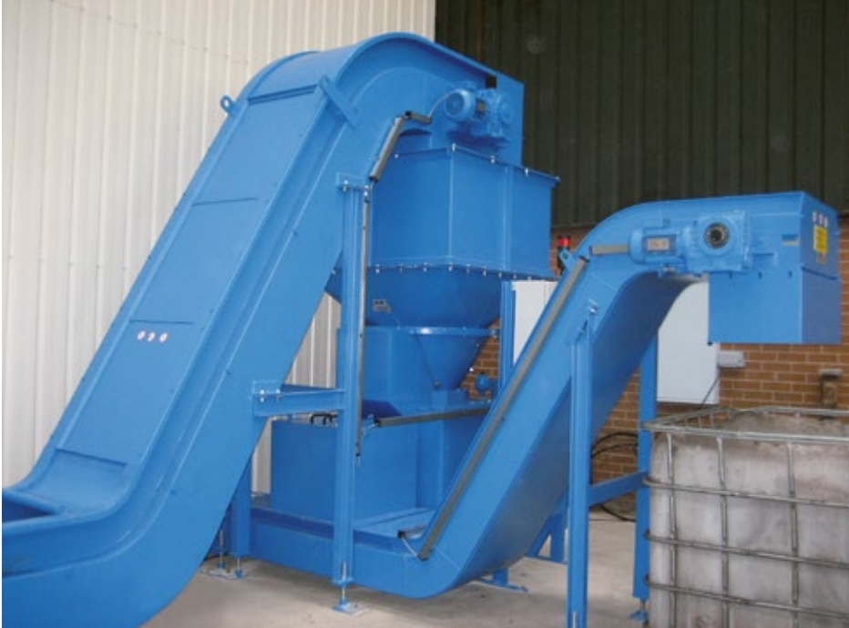
Swarf processing system with VBU centrifuge and swarf crusher
