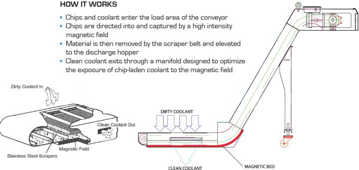
For dedicated cast or ductile iron applications, Mayfran recommends using an AT-Cleaner sidestream package in conjunction with the MagSep magnetic scraper conveyor. The AT-Cleaner will help remove a high percentage of the sludge forming super-fines from the coolant tank.
