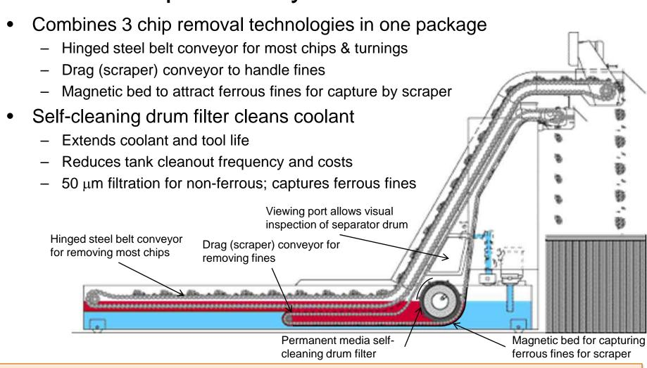
Handles the full range of chip, coolant, and material types
