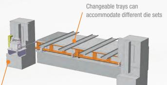
Press column mounting of shuffle drive motor is just one possibility that can be applied to provide easy access to the press
